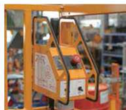
▷ Joystick provides precise and simultaneous travel control
